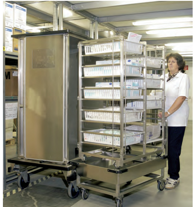
AGV transport cart during assembly at the central store in combination with the Hammerlit-Shuttle-System. Pictures taken at the university hospital in Leipzig, Germany
