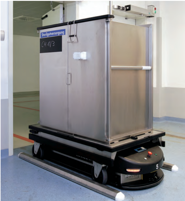
AGV transport cart is collected automatically
