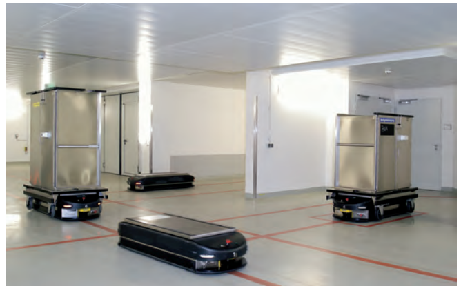
AGV transport units are routed automatically to their destination
